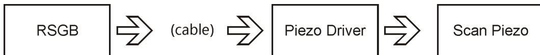
Figure 17. SASS signal path. Note that the PDC6N and PDC4N have a front connector XYZ IN.
